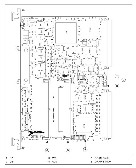
Figure 4-1. VME-MXI-2 Parts Locator Diagram
